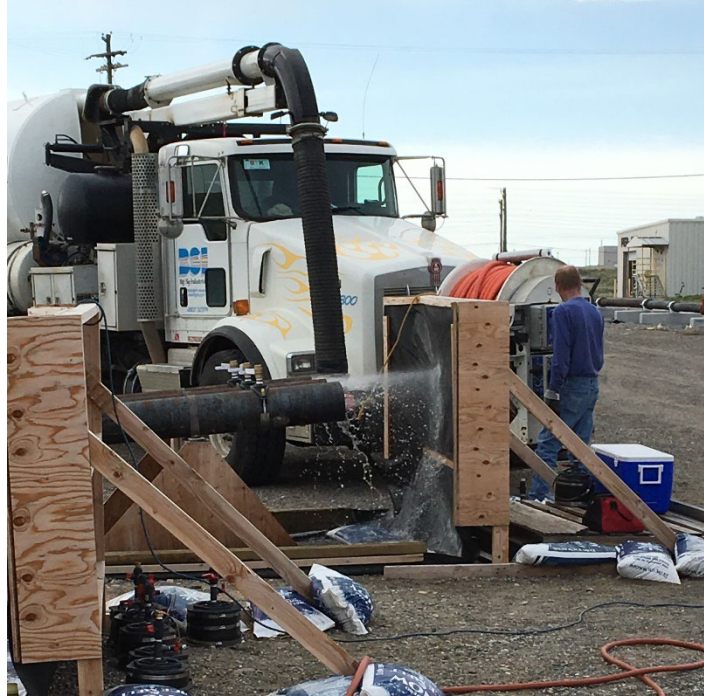
Figure 8: Water jet nozzle inserted into a pipe section.
