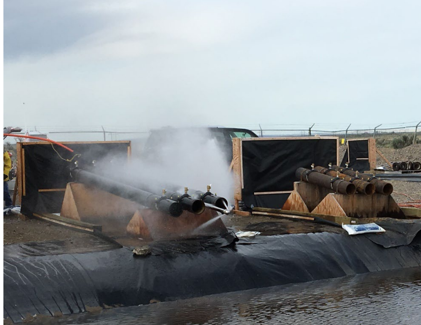
Figure 10: Jet sprayer nozzle exiting a pipe section.
