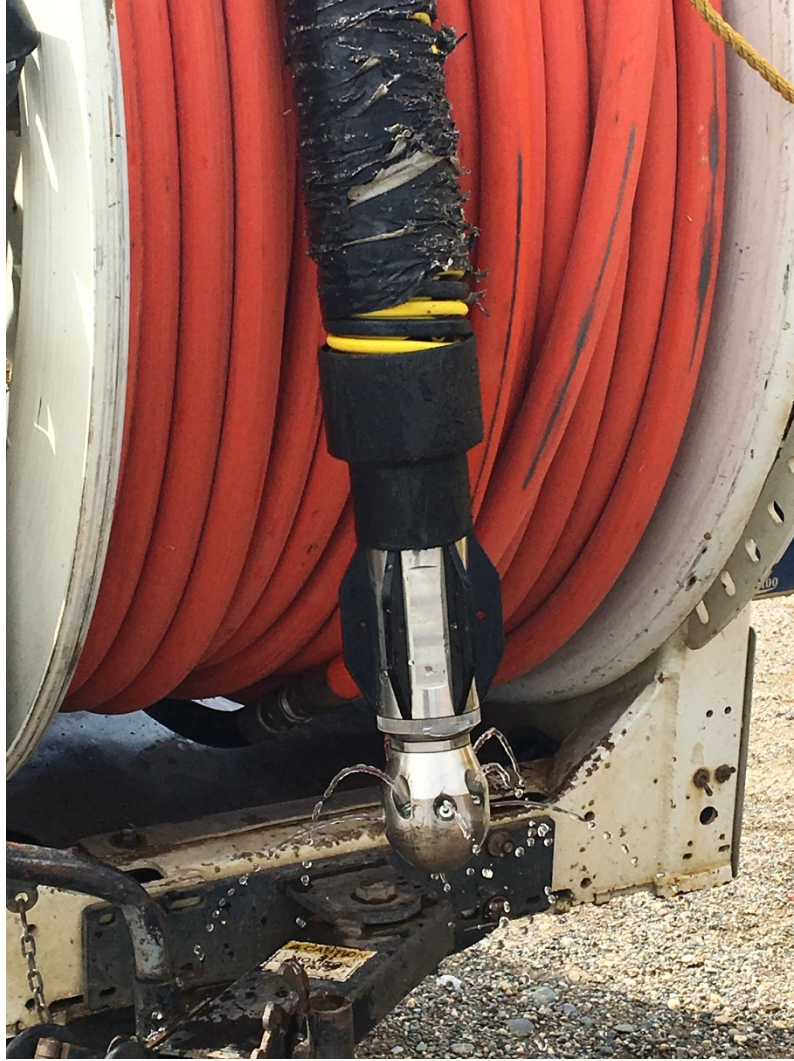
Figure 7: Water jet nozzle attached to the combination truck high pressure hose.
