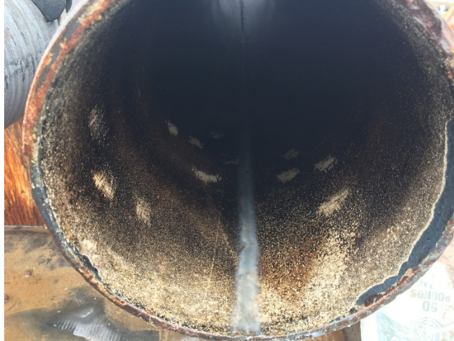
Figure 13: DragX coated pipe after curing overnight.
