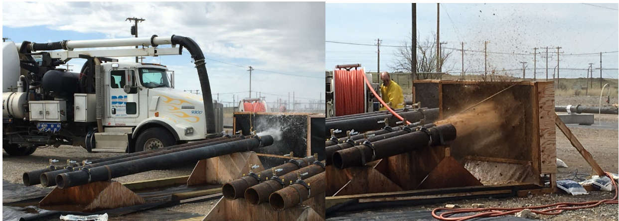
Figure 9: Spray coming out of a pipe section as the water jet nozzle travels down the pipe.
