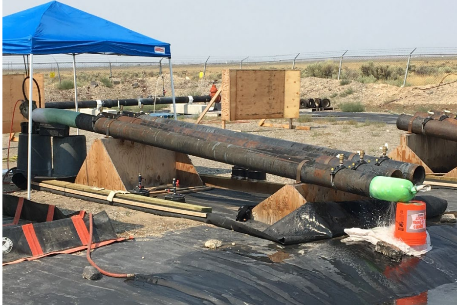
Figure 17: CIPP filled with hot water and in the process of curing.
