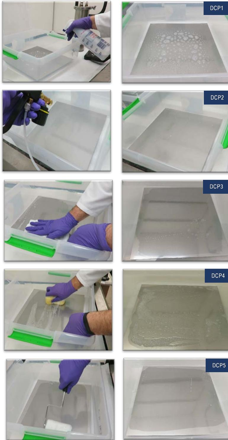
Figure 3-11. DCP1 through DCP5 application of decontaminant using various cleaning media and resulting appearance of the TC surface
