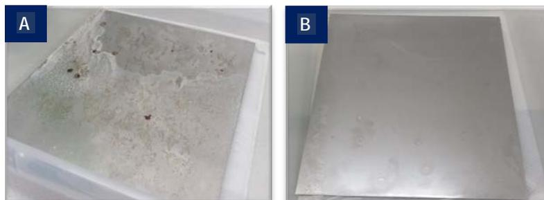
**Figure 5-7. Appearance of the material surface after multistep treatment with bleach (A) and EasyDecon® DF200 (B).**
