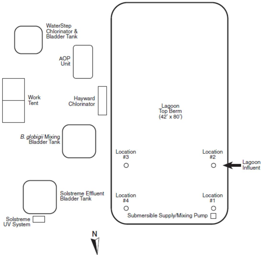
**Figure 5. Schematic layout for large volume water treatment technologies testing.**
