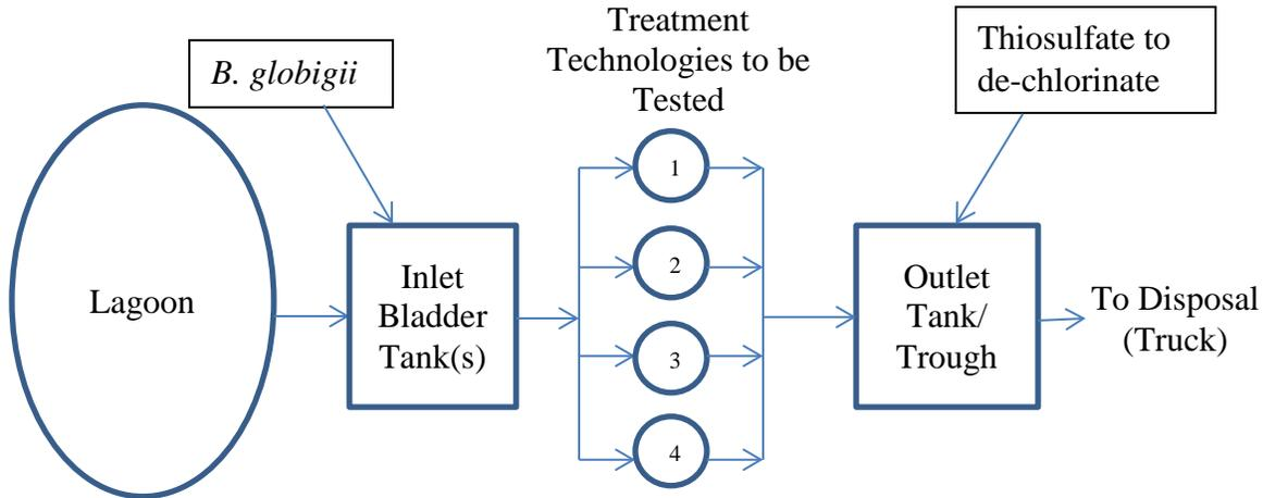
**Figure 3-2: Large Water Volume Testing Schematic**
