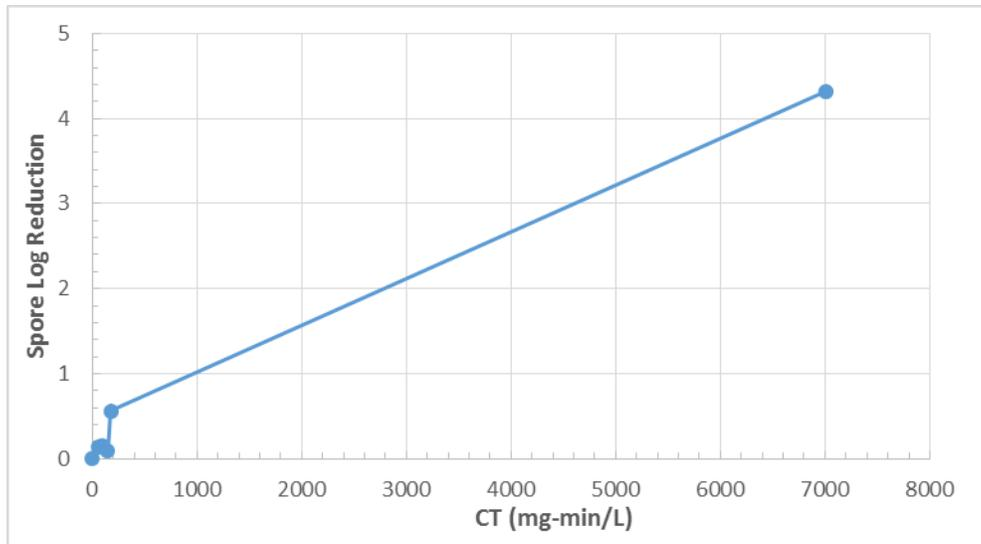
**Figure 28. The log reduction in spores during the Hayward experiment plotted against the Ct value (disinfectant concentration multiplied by time).**
