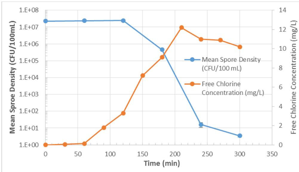
**Figure 25. Free chlorine concentration (orange) and *Bacillus globigii* spore (blue line) density over time in the WaterStep bladder tank.**
