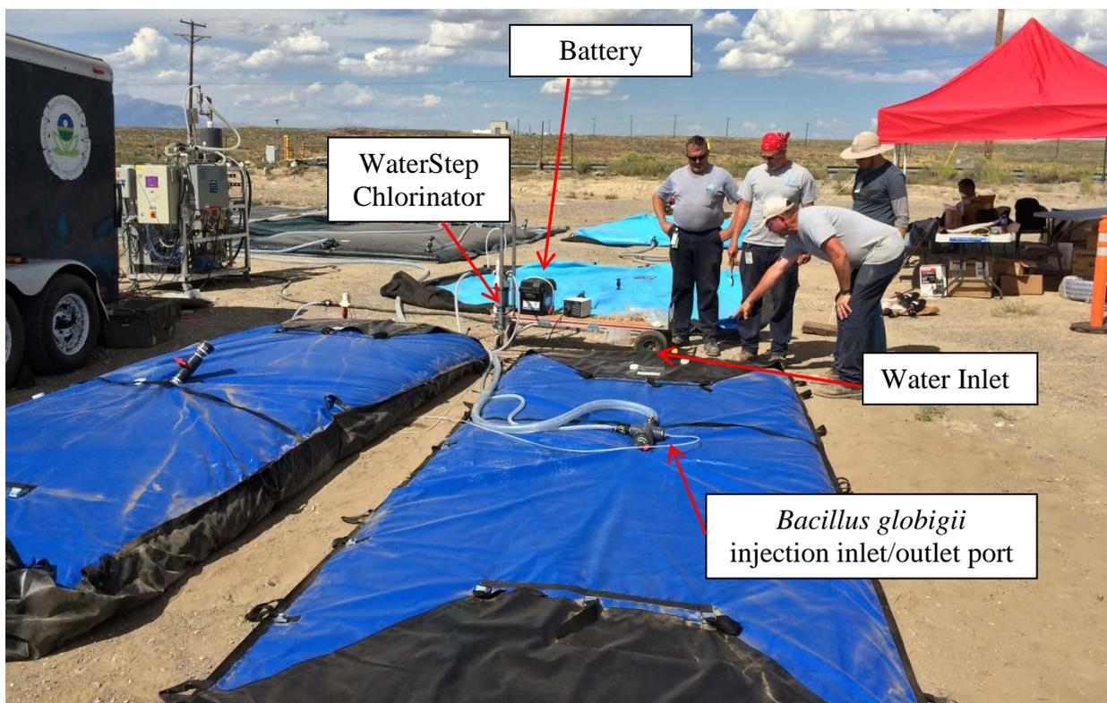
**Figure 13. WaterStep Chlorinator System bladder tanks (dark blue).**
