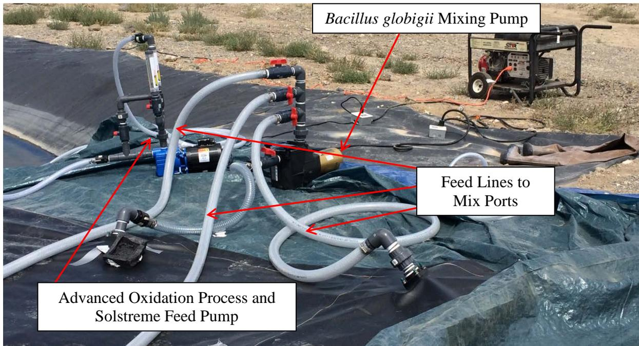
**Figure 9. Inlet bladder tank and mixing.**
