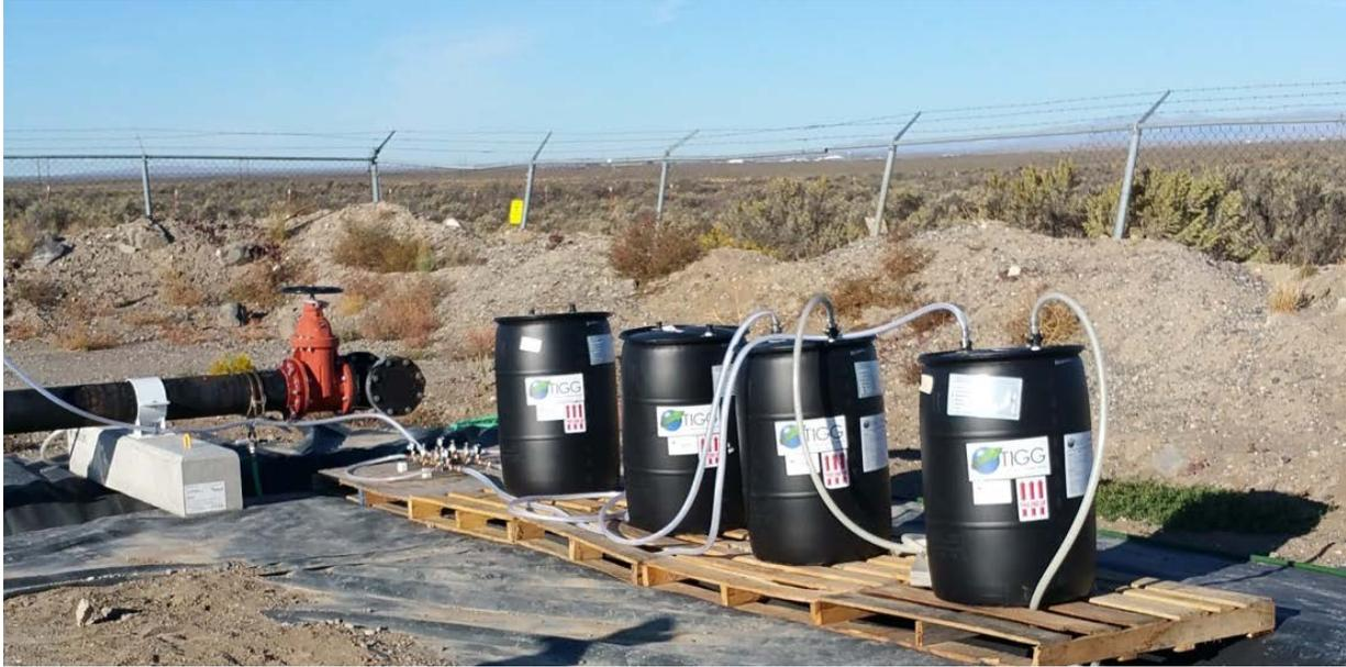
**Figure 20. Effluent oil capture treatment train.**
