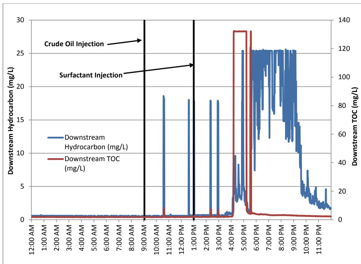
**Figure 30. Online total organic carbon (TOC) and hydrocarbon sensor data during the crude oil contamination and surfactant decontamination (9/21/2015).**
