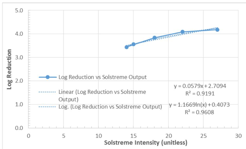
**Figure 24. Spore log reduction for Solstreme UV treatment vs. UV output intensity. Solstreme output intensity is a proprietary, unitless measure of UV intensity. Both linear and logarithmic best fit lines are shown.**
