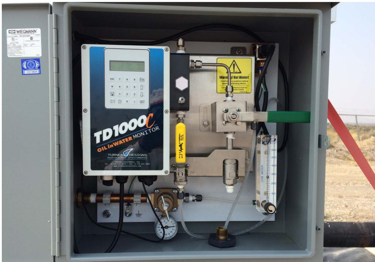
**Figure 19. Turner TD1000C Oil in Water Monitor.**
