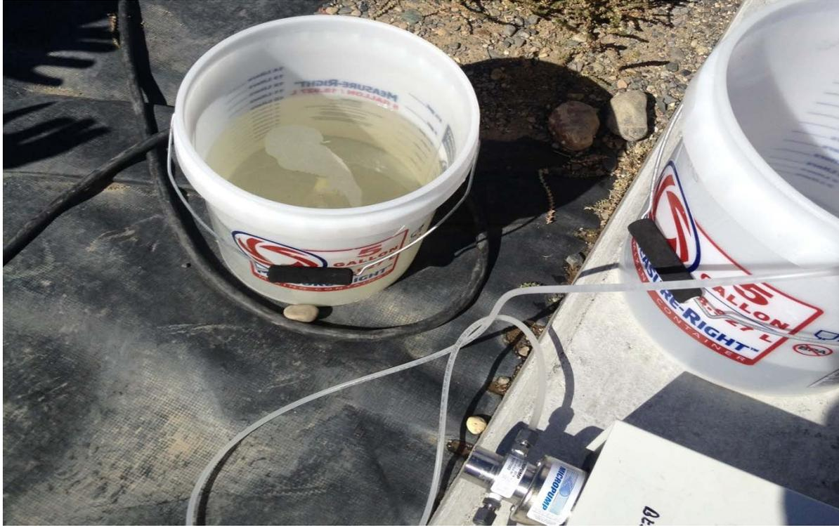
**Figure 6. Prepared crude oil subnatant for Water Security Test Bed injection.**
