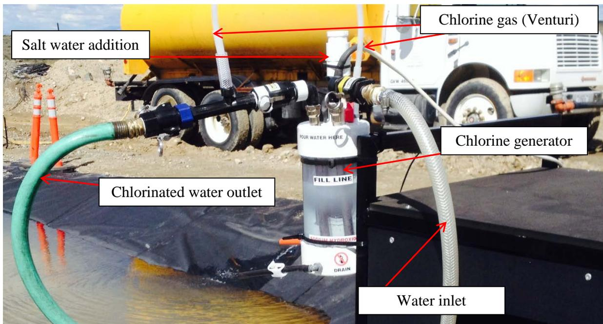
**Figure 14. WaterStep Chlorine Generator components.**
