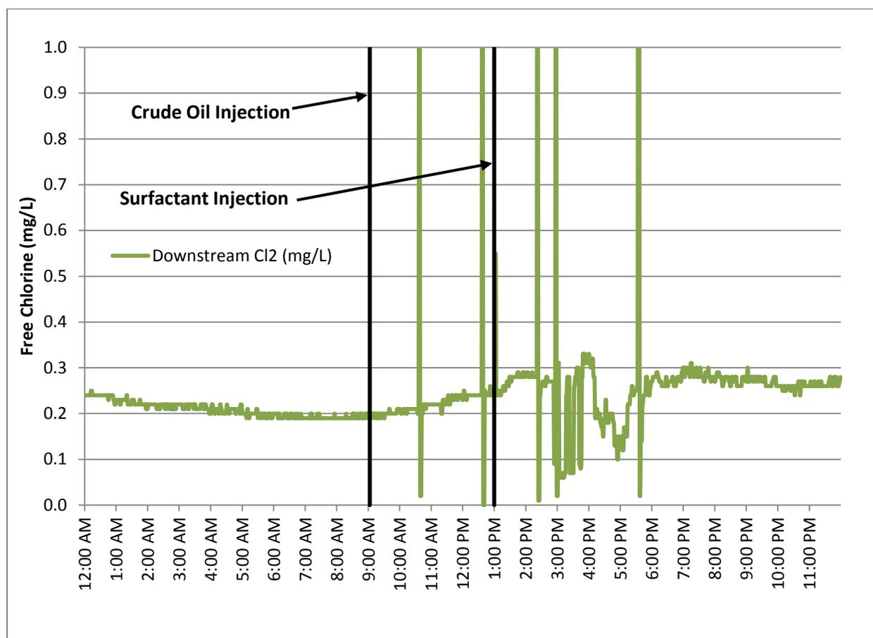
**Figure 31. Online chlorine sensor data during the crude oil contamination and surfactant decontamination (9/21/2015).**
