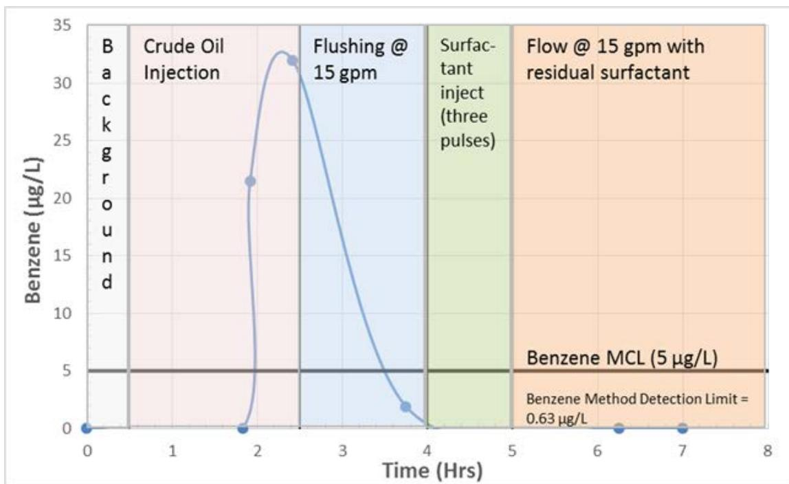
**Figure 29. Benzene concentration in the Water Security Test Bed bulk water.**
