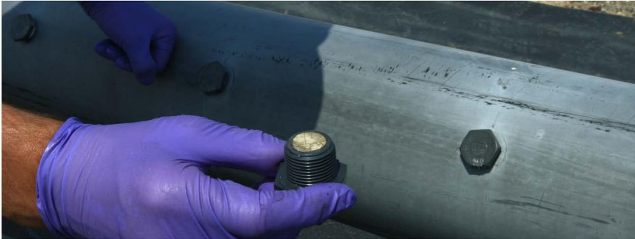
**Figure 8. Extracted pipe coupon.**
