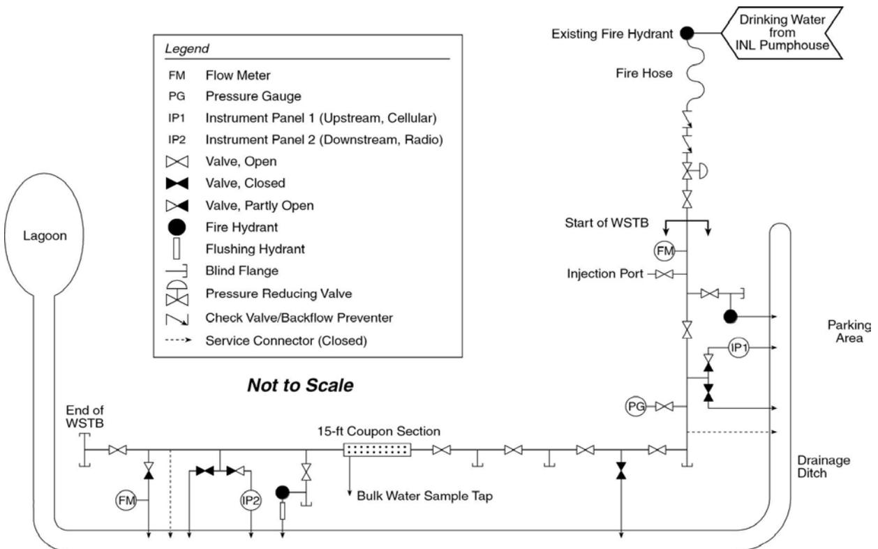
**Figure 3-1: Schematic Overview of WSTB**
