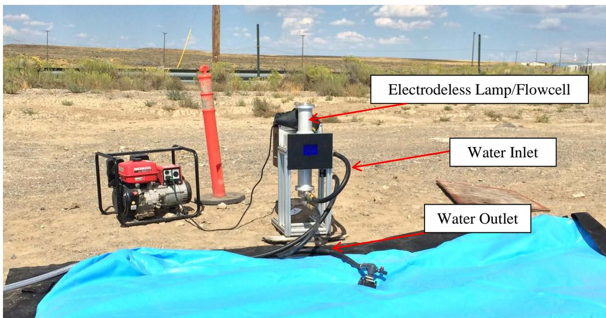
**Figure 12. Solstreme™ UV System and effluent bladder tank (blue object in front of the UV system).**
