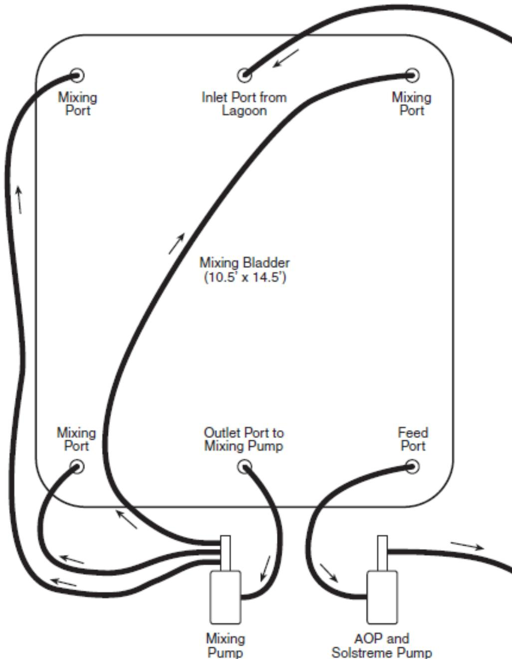
**Figure 10. Schematic depiction of the inlet bladder tank mixing process.**
