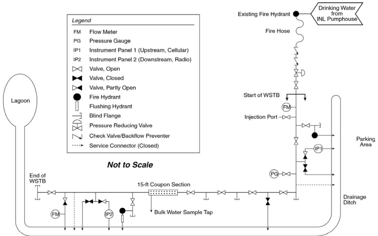
**Figure 1. Schematic overview of Water Security Test Bed.**
