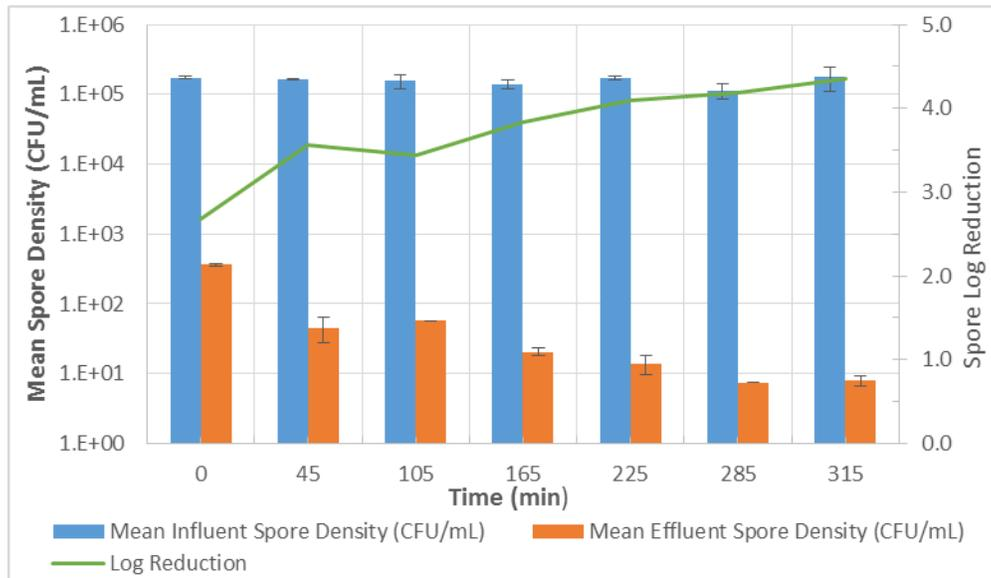
**Figure 23. Treatment performance of the Solstreme over the course of 5.5 hrs. Blue and orange bars represent the mean spore density in the Solstreme influent and effluent, respectively. The green line represents log reduction, or the amount of inactivation occurring at each sampling point. Error bars represent the range between duplicate samples taken at each time point.**
