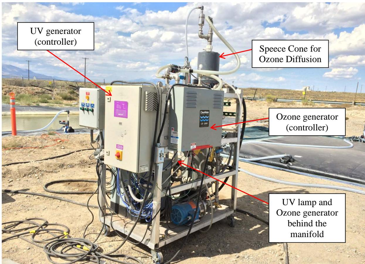
**Figure 11. Advanced Oxidative Process System and influent/mixing bladder tank (black object to the right of the system).**
