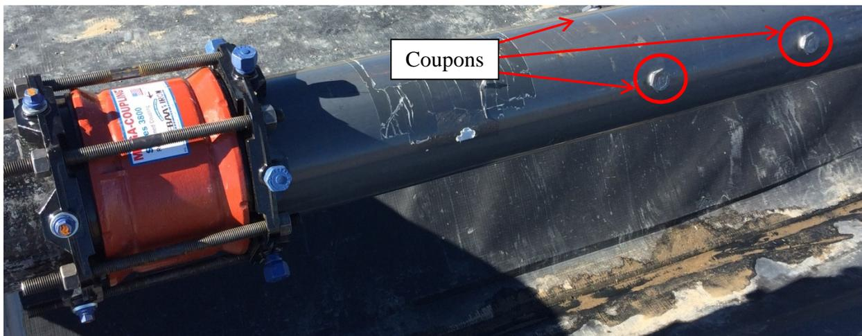
**Figure 7. Removable 15-foot PVC coupon section.**
