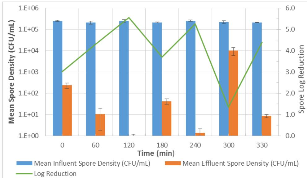
**Figure 22. Treatment performance of the Advanced Oxidation Process trailer over the course of 5.5 hrs. Blue and orange bars represent the mean spore density in the AOP trailer influent and effluent, respectively. The green line represents log reduction, or the amount of inactivation occurring at each sampling point. Error bars represent the range between duplicate samples taken at each time point.**
