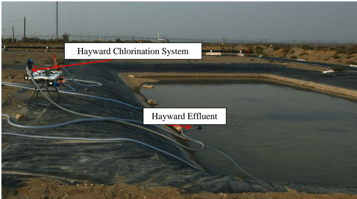
**Figure 16. Hayward Saline C™ 6.0 Chlorination System setup on a table.**
