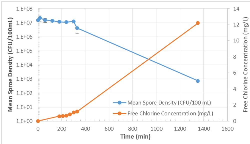
**Figure 27. Free chlorine concentration (orange) and *Bacillus globigii* spore (blue line) density over time in lagoon water (~5,000 gal) during disinfection with the Hayward treatment unit.**
