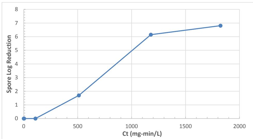
**Figure 26. The log reduction in spores during the WaterStep experiment plotted against the Ct value (disinfectant concentration multiplied by time).**
