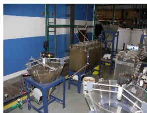
Activated sludge experimental set-up: assessing how contaminants travel through waste water treatment systems
