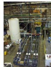
Waste water test bed: assessing persistence of contaminants on sewer infrastructure
