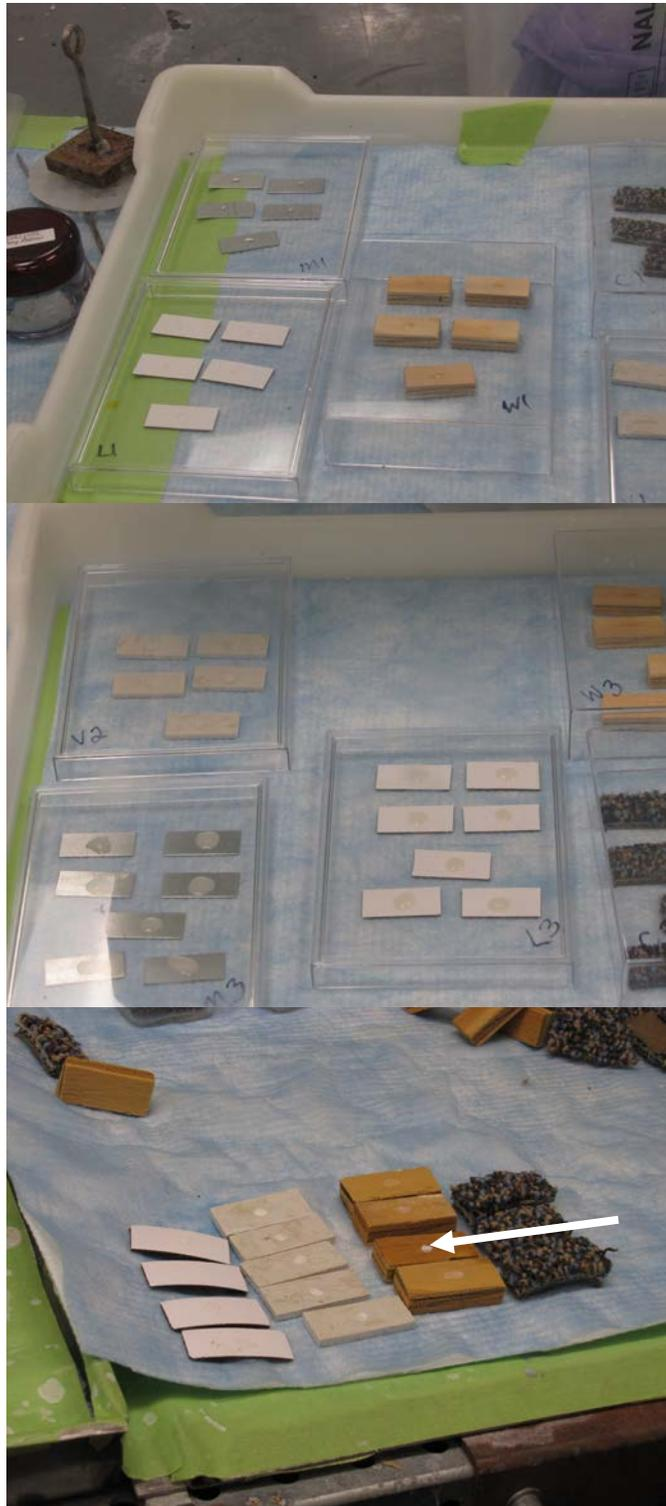
**Figure 2. Coupons before application of CWA (top), during DEFENZ™ VX-G decontamination (center) and after enzymatic decontamination (bottom) with residual plastic thickener from TGD visible, e.g., as shown by arrow.**
