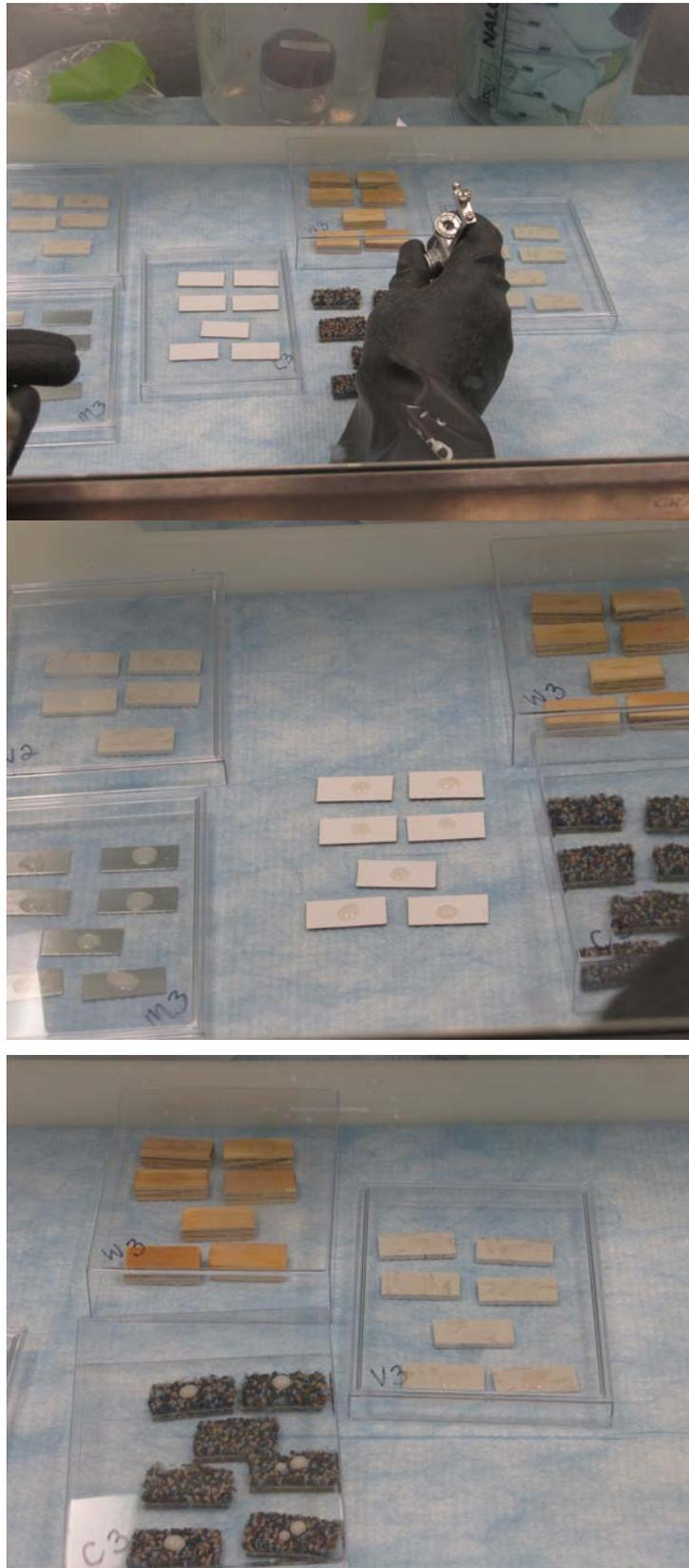
**Figure 3. Coupons during application of VX (top) and during DEFENZ™ VX-G decontamination (center, bottom).**
