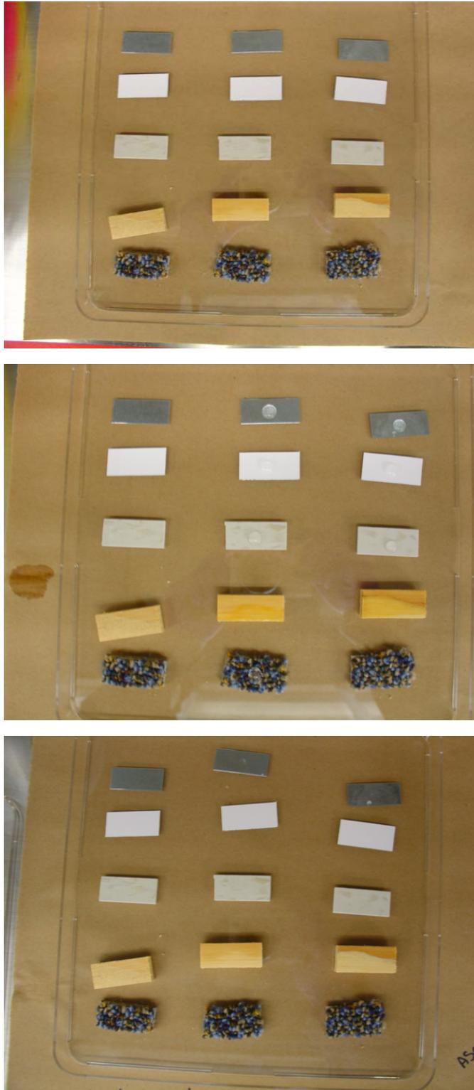
**Figure 4. Coupons before application of HD (top), during DEFENZ™ B-HD decontamination (center) and 48 hours after decontamination (bottom).**
