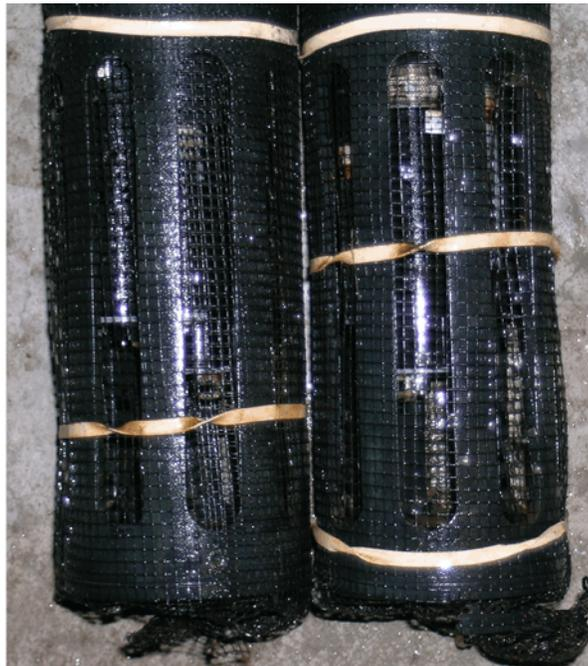
**Figure 6-4. 6600 EDS After Freshwater Deployment**
