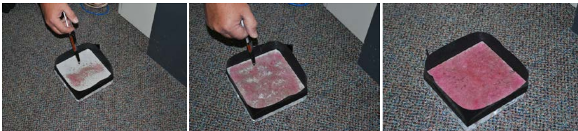
Figure 3-1. Demonstration of contaminant application technique.
