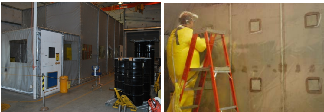
Figure 3-2. Containment tent: outer view (left) and inner view with test stand containing contaminated coupons (right).
