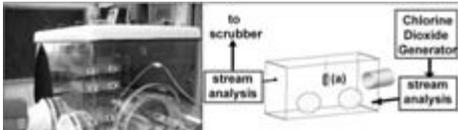
Photograph shows chamber loaded with concrete coupons. Coupon positions marked.
