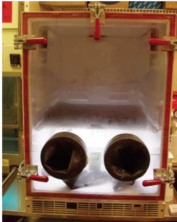
Figure 2-2. Refrigerator configured with ultraviolet-A/B lamps
