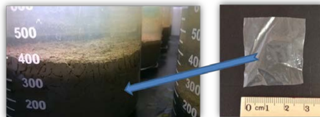
Figure F-14. Laboratory bioaccumulation experiment using the freshwater oligochaete, L. variegatus with polyethylene passive samplers inserted in exposure beakers to measure freely dissolved porewater concentrations of PAHs and PCBs.
