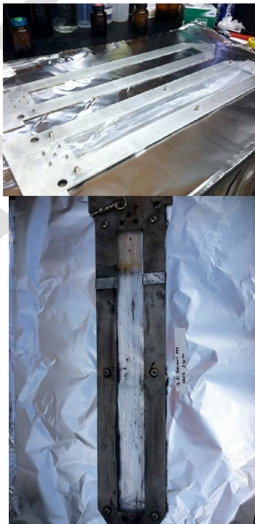
Figure F-10. Assembly of samplers prior to deployment (top), and a sampler after retrieval (bottom), showing the sediment/water interface right above the white tape mark. The total length of the LDPE window was ~50 cm.
