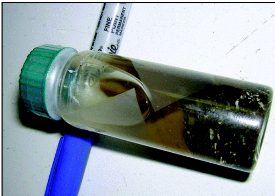
Figure 2-1. Polyoxymethylene passive sampler strip in a laboratory vial (40 mL) for an ex situ deployment in a water-sediment slurry for sampling porewaters (image provided by SB Hawthorne (University of North Dakota, Grand Forks, ND, USA)).
