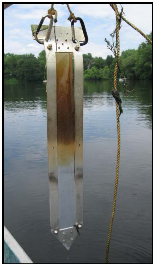
Figure 4-5. Photograph of LDPE in an aluminum frame after deployment in a freshwater lake sediment. The lower portion of the LDPE, which still appears transparent, was embedded below the sediment-water interface; in contrast, the LDPE in the lake-bottom water was coated in material that may affect target contaminant uptake rates in the LDPE.
