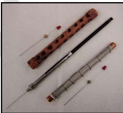
Figure 3-4. SPME fibers configured to be wrapped in fine stainless steel mesh and fit inside copper (or stainless steel) tubes for in situ deployment in the water column or in sediments. SMPE fiber shown are extended from syringes during deployment (based on Maruya et al. 2009).
