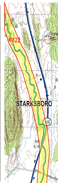
Figure 4-3 Lewis Creek in Vermont is a watershed with very high recovery potential. Tier 1, 2, and 3 data are used to identify the reach M22 corridor as a priority for a conservation easement to protect sediment/nutrient storage processes.
