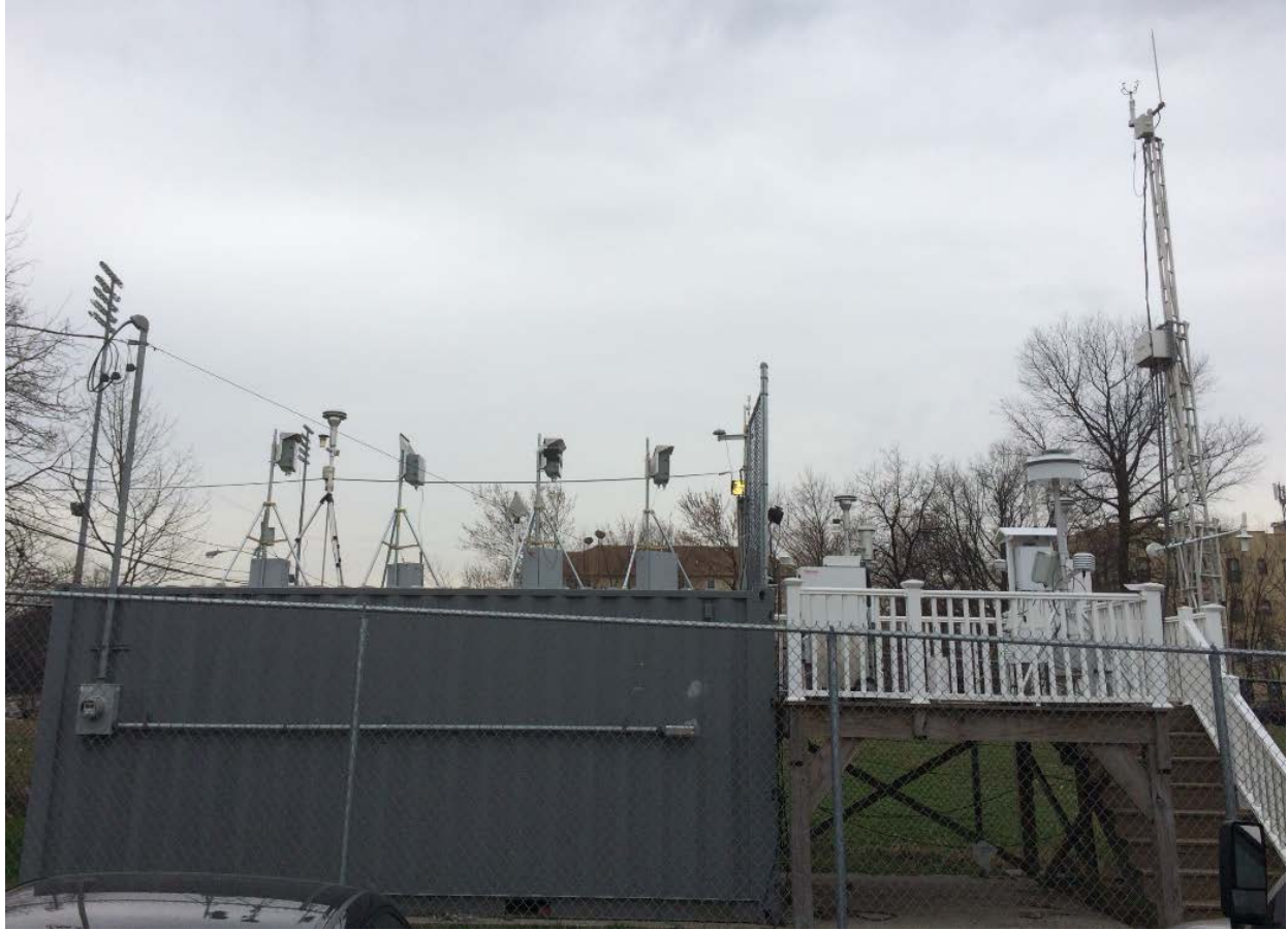
Figure 2-3. Four CSAM samplers were deployed on the roof of NJDEP's NCore station at the Clinton Avenue Firehouse in Newark, NJ.
