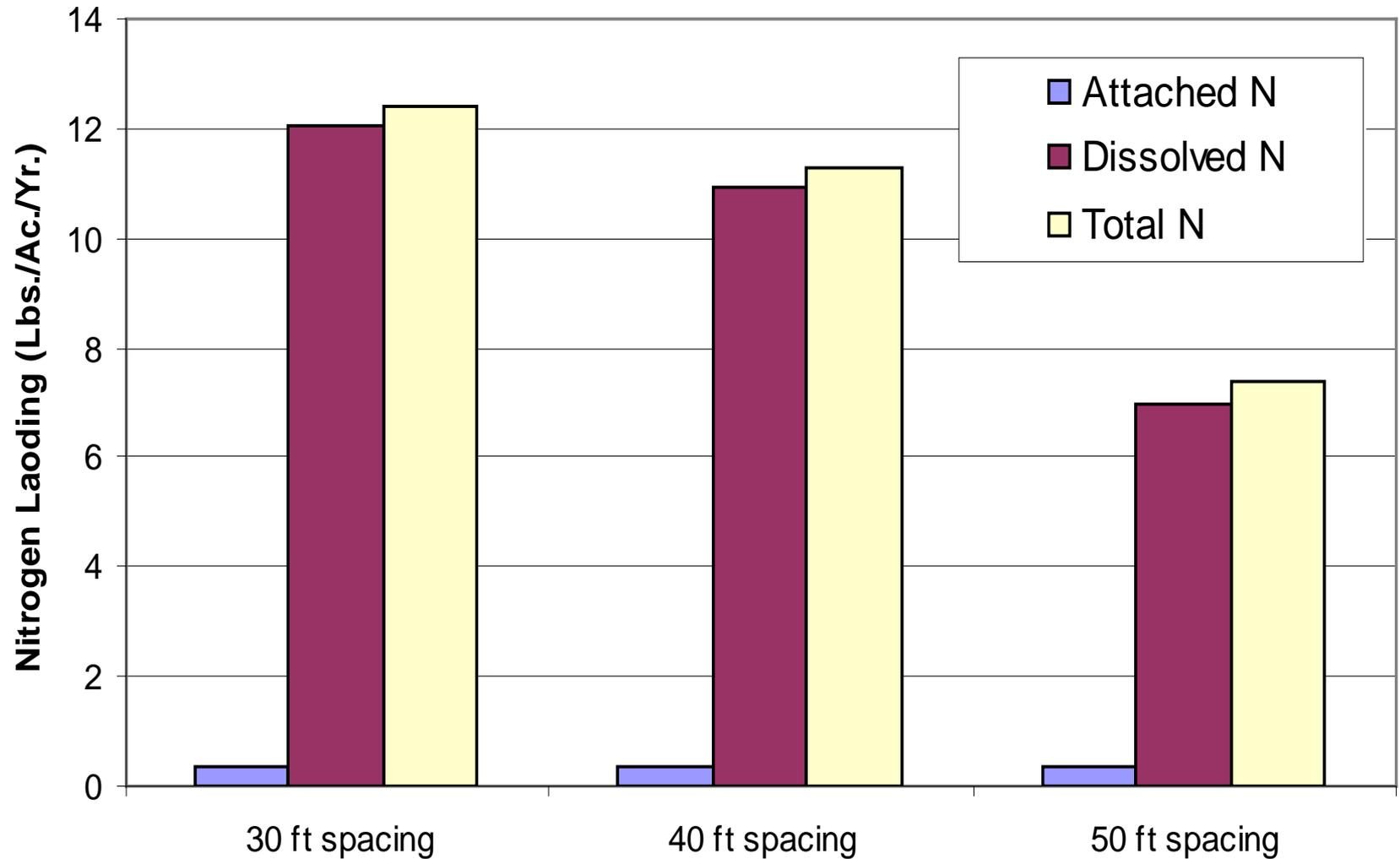
Effects of drain spacing on nitrogen loading (drains at 48" depth)
