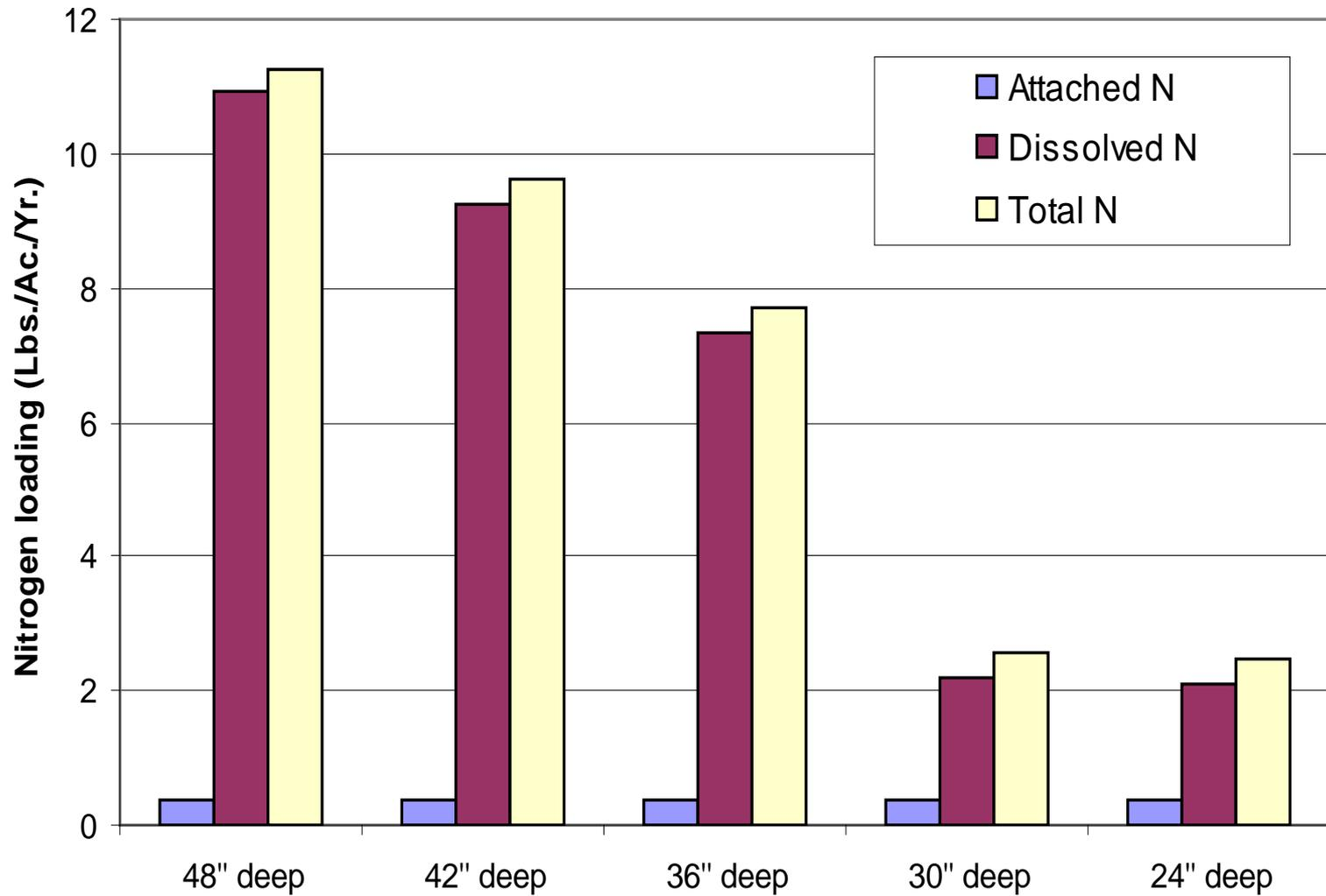
Effects of drain depth on nitrogen loading (40 ft drain spacing)
