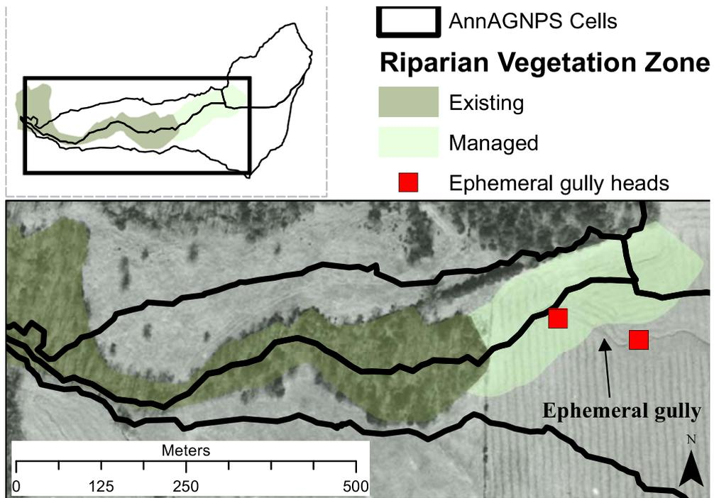
**Figure 8.** Simulated scenarios considered in the evaluation of the vegetation type on the AnnAGNPS riparian buffer component estimation of sediment loads.
