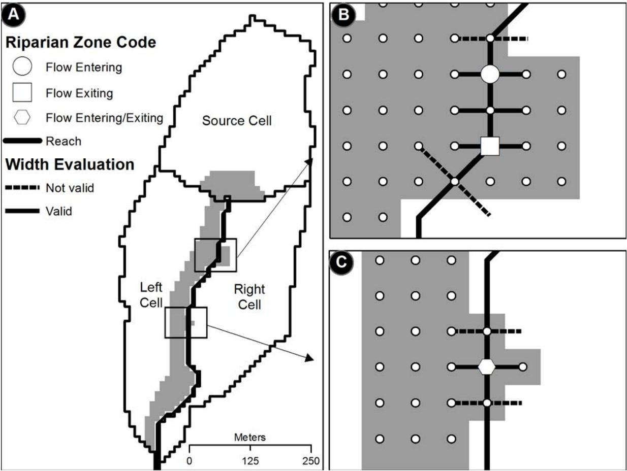
**Figure 6.** Schematic of GIS analysis performed for the estimation of sediment trapping efficiency when reaches go through riparian vegetation zones.
