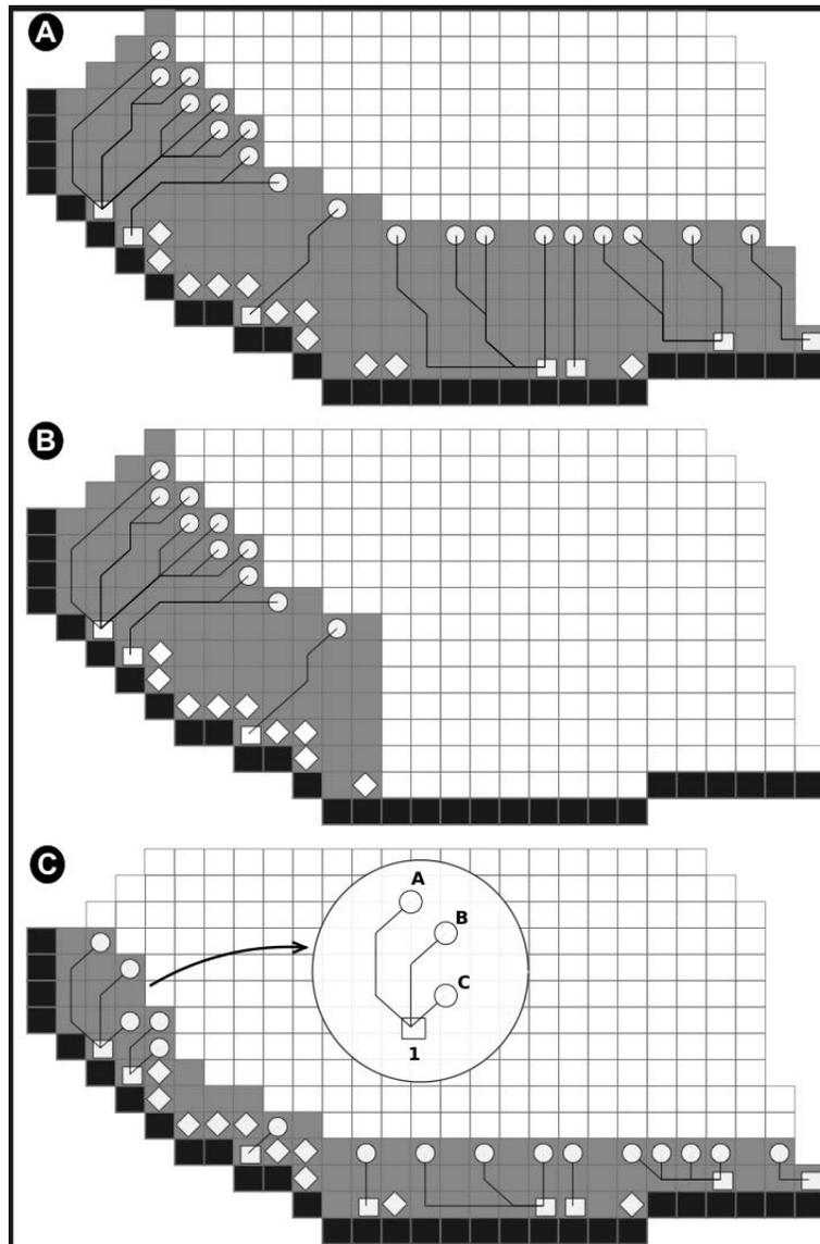
**Figure 4.** Distinction of downstream edge raster grid cells between flows that enter from outside the filter strip (squares represent the most downstream raster grid cell of these flows) and flows that begin inside the filter strip (diamonds represent the most downstream raster grid cell of these flows) for a riparian zone extent completely across the cell area that connects to a reach (A), partially across the cell (B), and is completely across the cell area and with reduced width (C).
