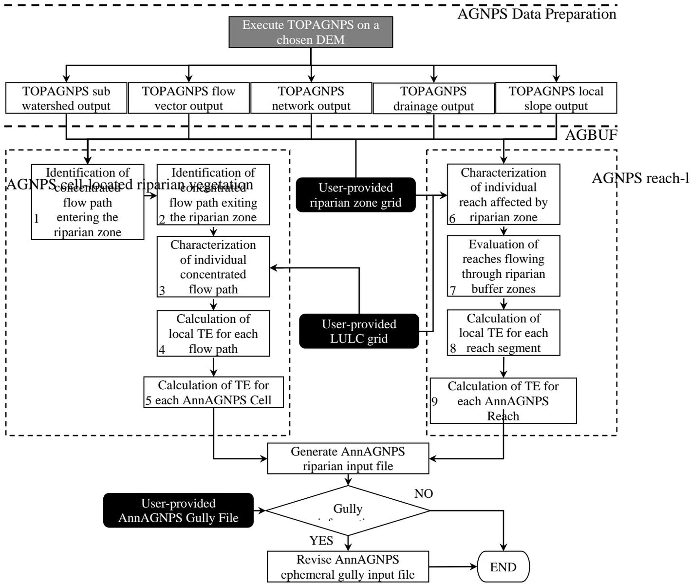
**Figure 2.** Schematic of the steps performed by the AGNPS riparian buffer component to estimate the effect of riparian vegetation on sediment loads for individual AnnAGNPS cells and reaches. Filled boxes indicate user-provided input information.
