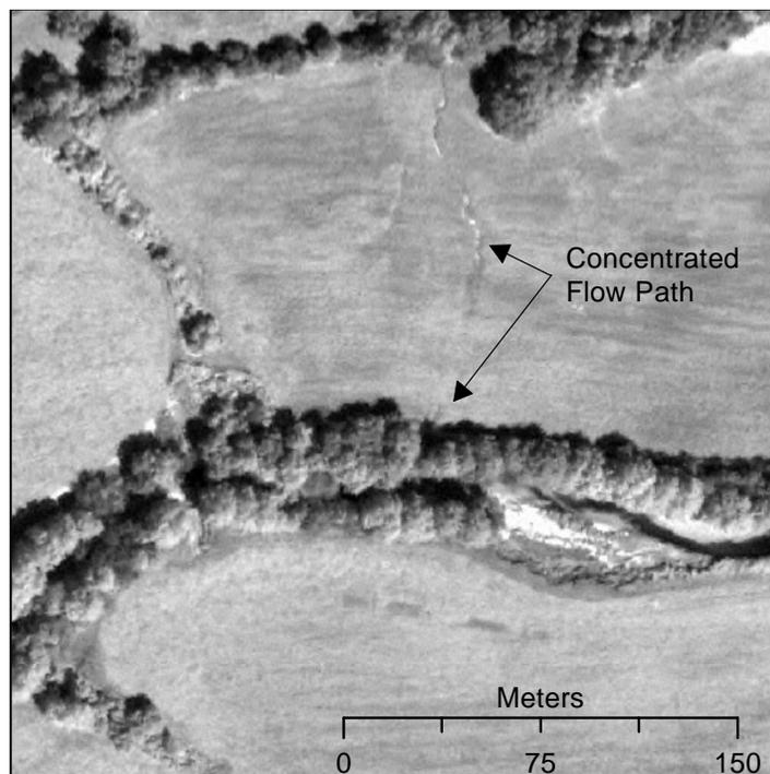
**Figure 5.** Aerial view of concentrated flow path “short-circuiting” the riparian vegetation buffer. Concentrated flows with high energy as result of steep slopes and/or large drainage area tend to sustain high velocities reducing, or even vanishing, the sediment trapping efficiency of riparian vegetative filter strips.
