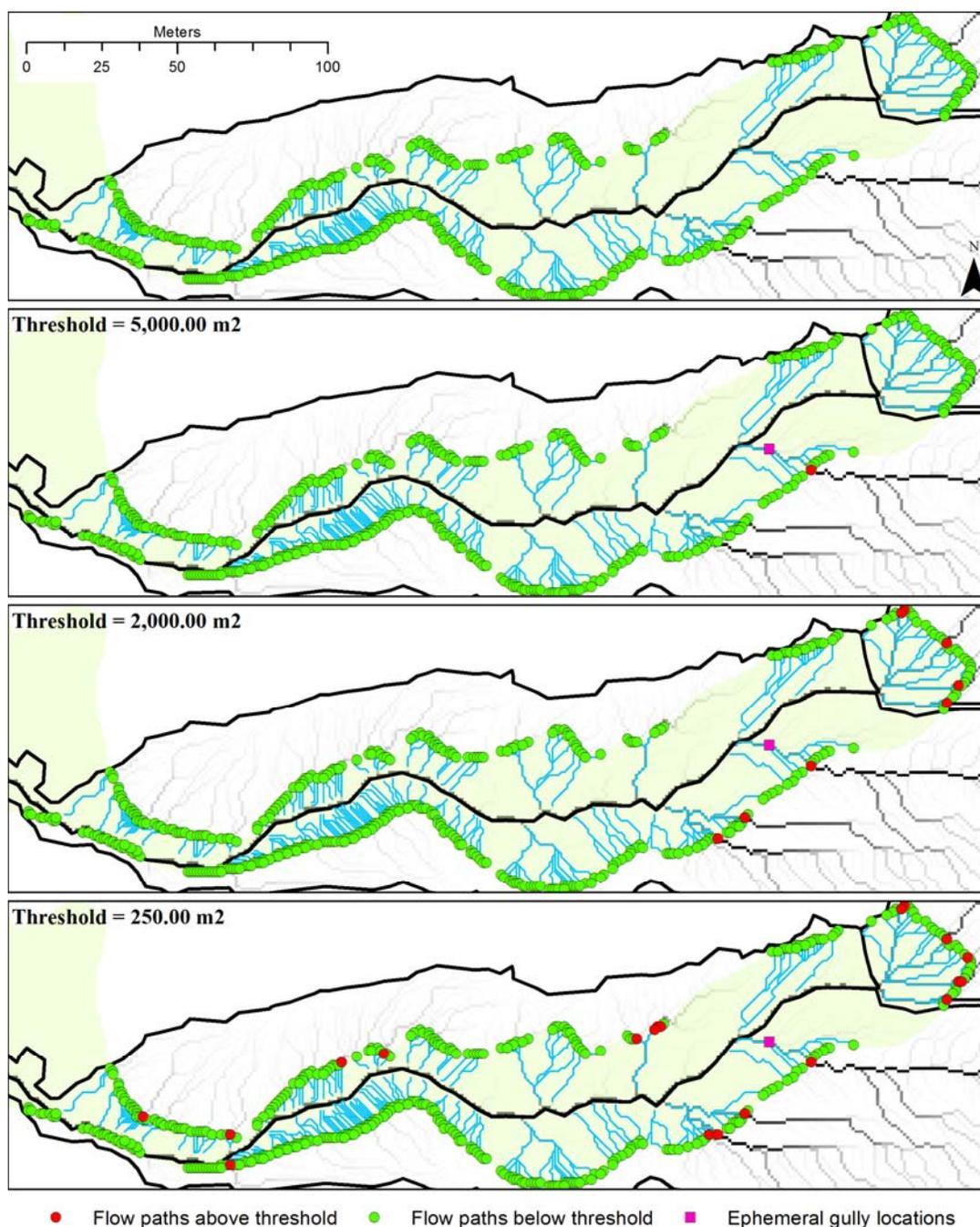
**Figure 10.** Simulated scenarios considered in the evaluation of the presence of concentrated flow paths with high energy (short-circuits) on the AnnAGNPS riparian buffer component estimation of sediment loads.
