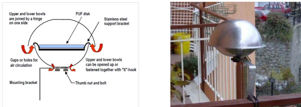
Figure S2. Schematic representation of the PUF disk sampler and photo of a PAS deployed.
