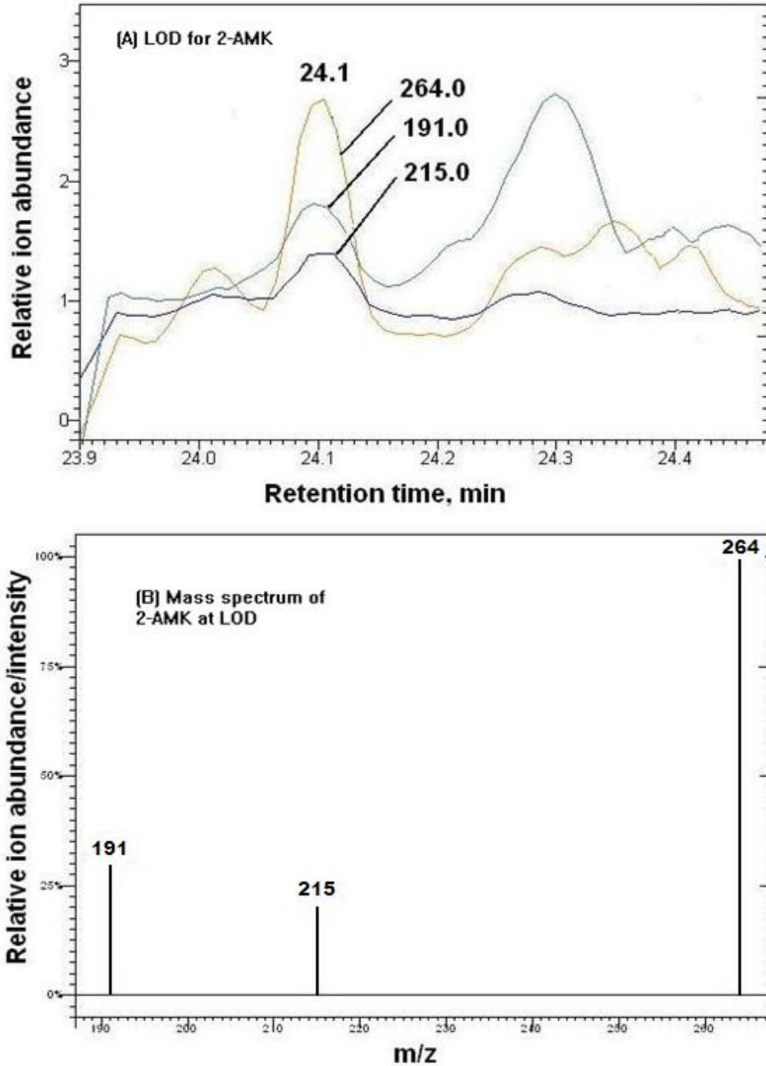
Figure 2. Identification of 2-AMK at LOD level, (A) GC-SIM-MS ions chromatogram and (B) the mass spectrum of the peak eluting from a capillary column at retention time 24.1 min. The GC-MS operating conditions are given in section 2.8.
