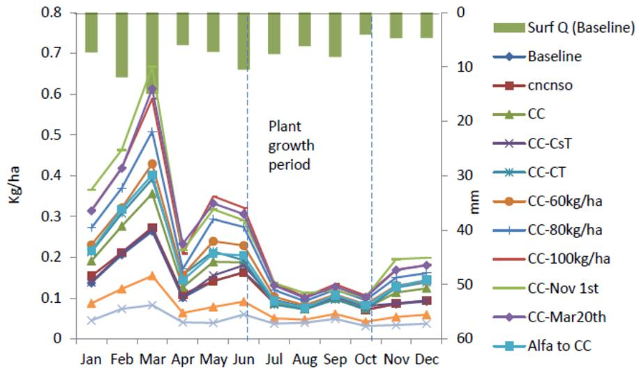
**Figure 6:** Monthly average TP loss at the watershed outlet from different crop management alternative scenarios
