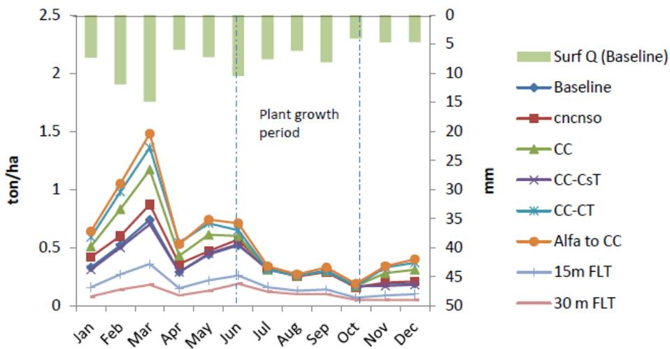
**Figure 5:** Monthly average sediment loss at the watershed outlet from different crop management alternative scenarios
