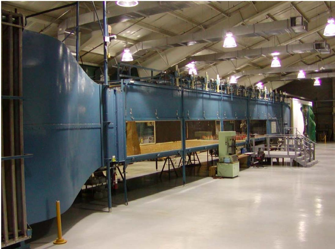
**Figure 6-2. The Fluid Modeling Facility houses the Division's meteorological wind tunnel used to study the effect of roadway configuration and wind direction on near-road dispersion.**
