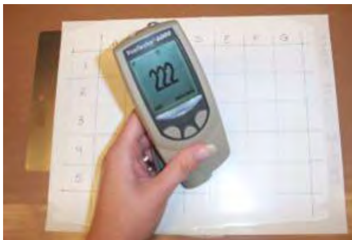
Figure 5. Marked paint film being measured for thickness.
