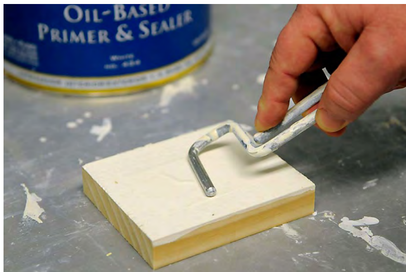
Figure 9. Smoothing out paint film after allowing time for the primer to partially dry.
