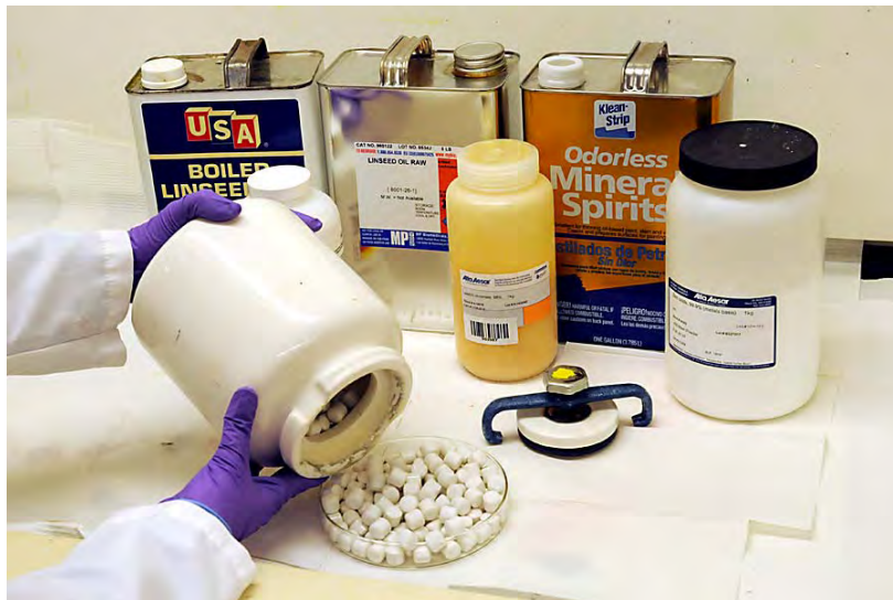
Figure 3. Ball mill jar with grinding media along with principal ingredients of paint.
