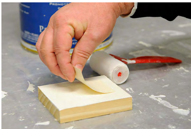
Figure 8. Placing leaded paint film on wood substrate coated with primer to serve as adhesive.
