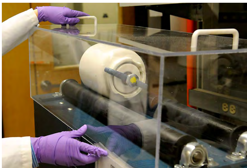
Figure 1. Ball mill being covered with safety shield to prevent injury from rollers.
