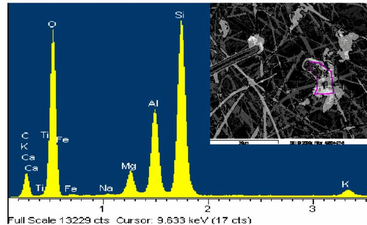
Figure C-2b. Clay particles on Subject 2's Respicon Filter.
