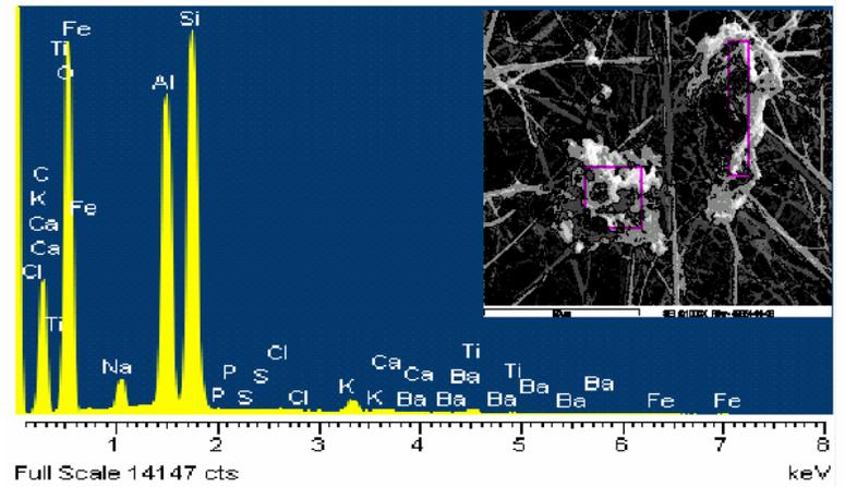
Figure C-4b. Clay particles on Subject 4's Respicon Filter.
