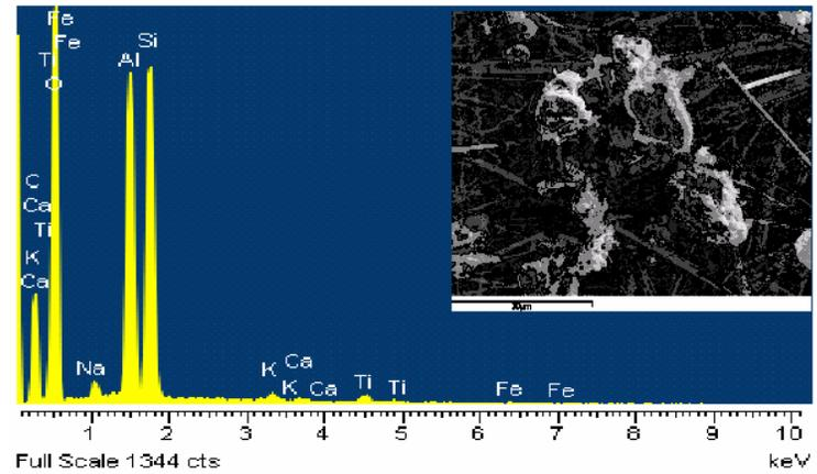
Figure C-7b. Clay particles on Subject 7's Respirator Filter.
