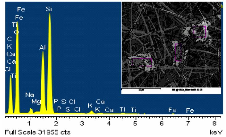
Figure C-3b. Clay particles on Subject 3's Respicon Filter.
