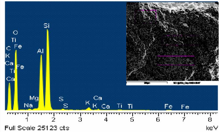
Figure C-3a. Sample of clay used by Subject 3.
