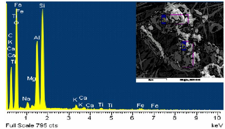
Figure C-6b. Clay particles on Subject 6's RespiCon Filter.
