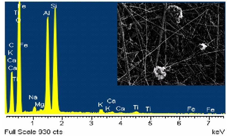
Figure C-5b. Clay particles on Subject 5's RespiCon Filter.
