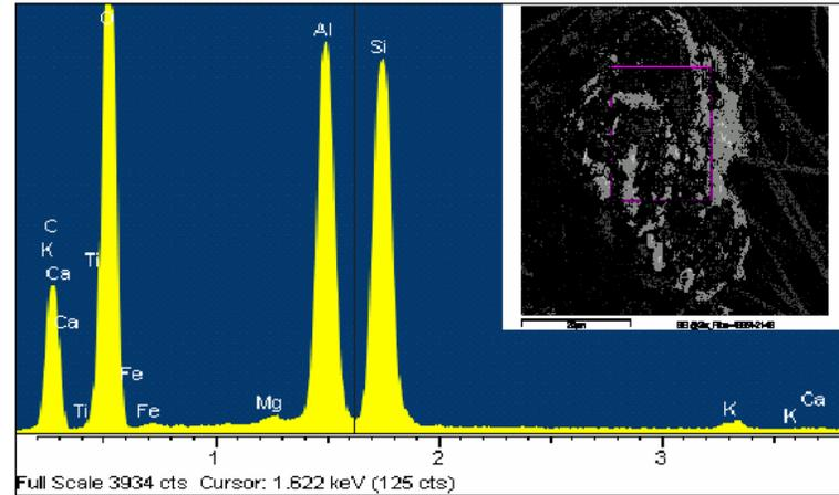
Figure C-1b. Clay particles on Subject 1's Respicon Filter.
