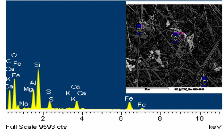
Figure C-8b. Clay particles on Subject 8's Respirator Filter.
