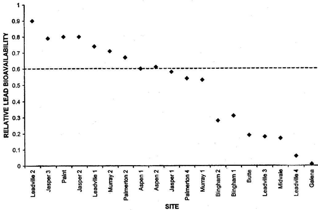
**Figure 4.** Swine feeding studies using 17 field soils contaminated with lead and two laboratory-prepared soils (paint in soil and galena in soil). The dashed line represents the 60 percent relative bioavailability used to set the national default value for absolute bioavailability of lead in soil used by EPA (Henningesen et al., 1998a).
