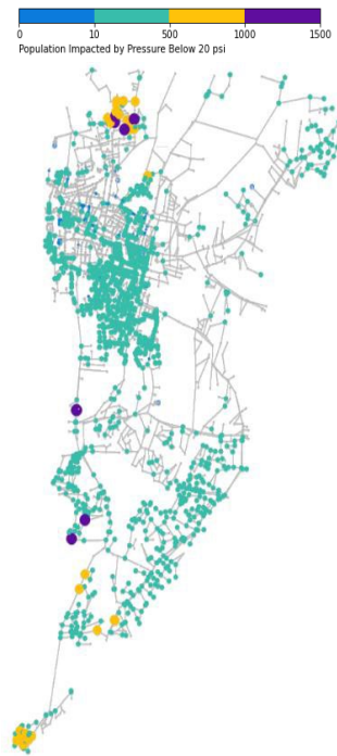
Figure 3. Poughkeepsie water network model with nodes highlighted with population impacted by reduction in water pressure due to increased demands from firefighting [modified from Chu-Ketterer et al., 2023a].
