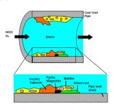
Over time, the iron surface is corroded and tubercles are formed
