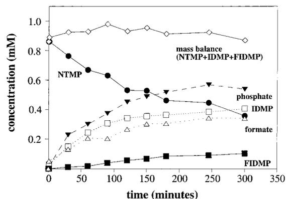
FIGURE 7. Loss of NTMP (0.85 mM) and appearance of four oxidation products as a function of time in the presence of  $0.85 \text{ mM } Mn^{II}$  (pH 7.1). To ensure constant  $[O_2(aq)]$ , the solution was constantly bubbled with laboratory air.
