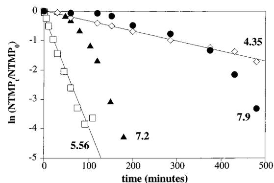
**FIGURE 2. Loss of NTMP as a function of time in the presence of 10 μM Mn<sup>II</sup> for 4 of the 18 runs shown in Figure 1.**
