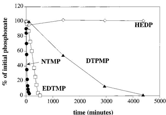
FIGURE 6. Loss of NTMP, EDTMP, DTPMP, and HEDP as a function of time in the presence of  $10 \mu M$   $Mn^{II}$  ( $10 \mu M$  ligand, pH 5.6).
