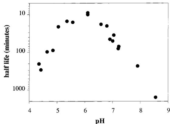
**FIGURE 1. Effect of pH on the half-life of 10 μM NTMP degradation following addition of 10 μM Mn<sup>II</sup>.**
