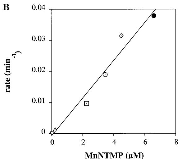
FIGURE 5. (A) Effect of  $O_2$ , Ca, Cu, and Zn addition on degradation of  $10 \mu M$  NTMP as a function of time at pH 7.0. The first experiment was conducted in an  $O_2$ -free glovebox. All other experiments were left open to laboratory air (0.21 atm  $O_2$ ). (B) First-order rate constants as a function of the sum concentrations of all possible Mn-NTMP complexes.
