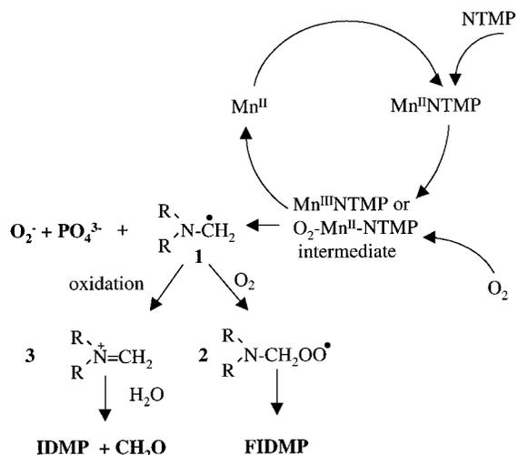
FIGURE 8. Tentative scheme of the degradation of NTMP in the presence of Mn<sup>II</sup> and O<sub>2</sub>.
