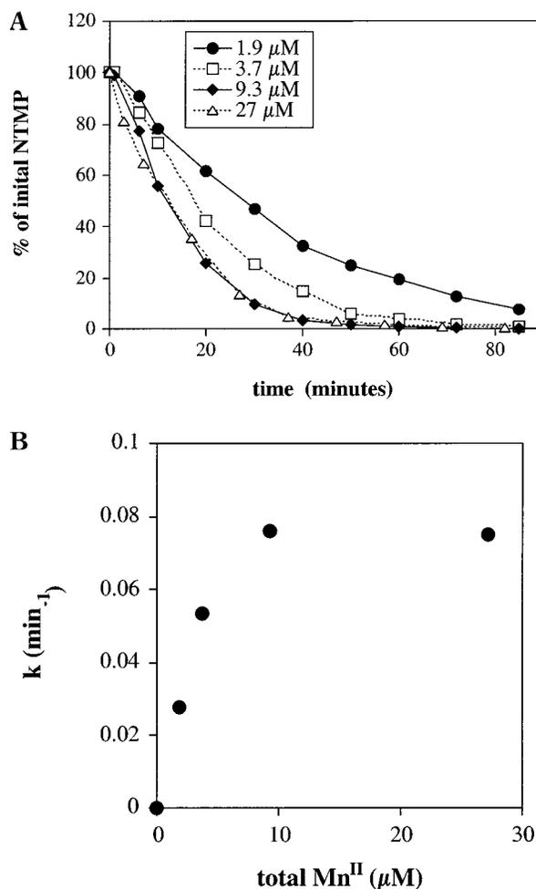
FIGURE 4. (A) Effect of  $\text{Mn}^{\text{II}}$  concentration on degradation of 10  $\mu\text{M}$  NTMP as a function of time at pH 6.0. (B) First-order rate constant as a function of the total added  $\text{Mn}^{\text{II}}$ .
